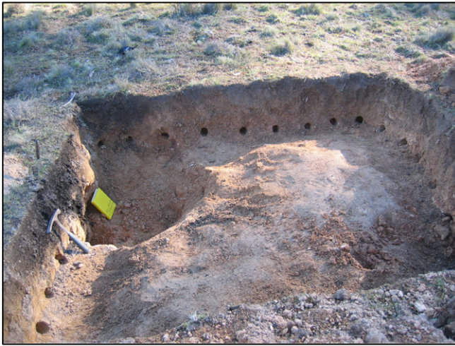
Fig. 3. Photograph (by AMH) of the FH 2-m pit. The west wall is on the far side of the pit from the camera. The direct push corer created the holes at the base of the walls, which are spaced 25 cm apart for bulk density analysis, as well as for the major and trace element analyses from every other hole shown. The floor of the 2-m \times 2-m pit was sampled with a 50-cm grid, where the outermost samples were at the edge of the pit (three samples on each edge between the two corner samples), and the nine inner samples were from the middle of the pit floor. The depression in the upper left quadrant is from the destruction of the pit floor by the collection of the first samples.
